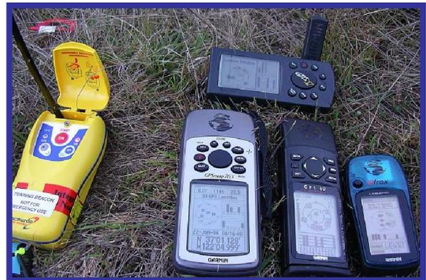
To record the number of satellites being received by the GPS and their signal strength, we used a waterproof Pentax OPTIO 33WR digital camera to photograph the GPS display. The
