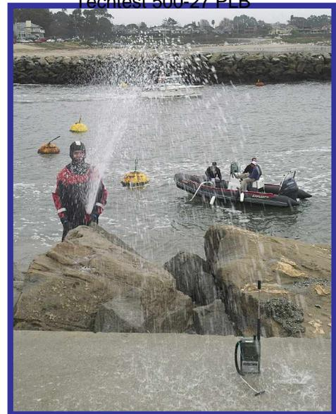
The RIB with water pump and an attached fire hose was located in the harbor channel adjacent to the jetty and a rescue swimmer used the hose to maintain a stream of water over the beacons that were set up on the edge of the jetty.
