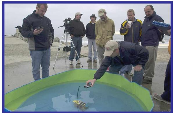
Maritime Scenario India – measuring 121.5 signal strength of McMurdo Fastfind Plus with base of the antenna submerged.
