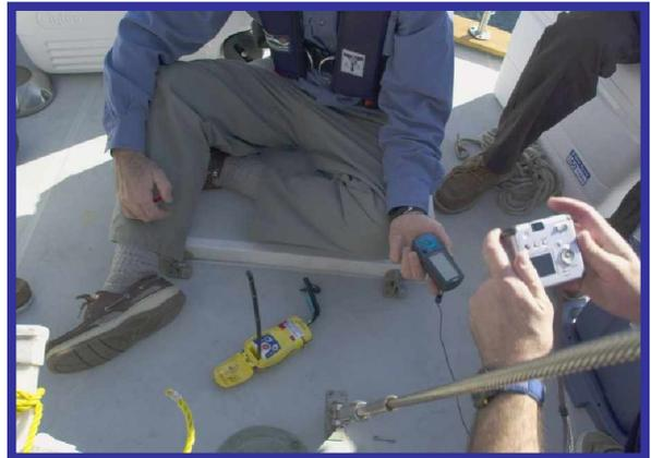
Maritime Scenario Alpha - aft deck of SV Willow, recording GPS satellites in view preparatory to activating McMurdo Fastfind Plus PLB
