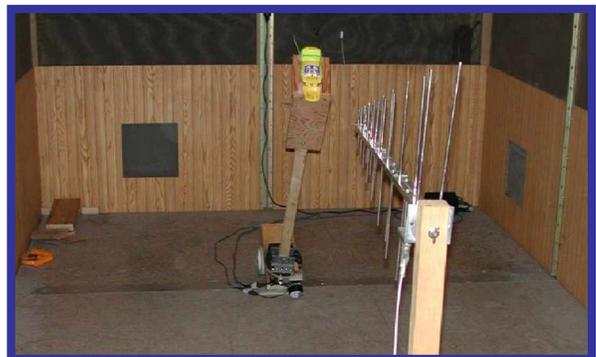
Test fixture for 40° measurements in RF screen room – McMurdo Fastfind Plus mounted
