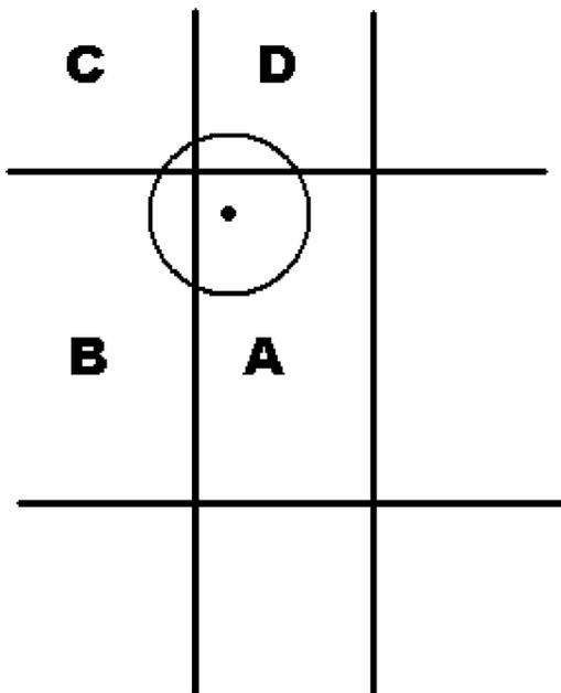
The beacon is located at the dot. The circle around it represents the GPS uncertainty. At latitude 37, the narrow side of the box is about 98.8 meters long, so this figure shows a GPS uncertainty of about 50 meters – which is a perfectly ordinary real-world figure.
