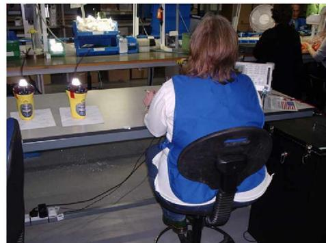
EPIRB testing (screened box on right)
