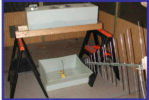
Test fixture for rain test
