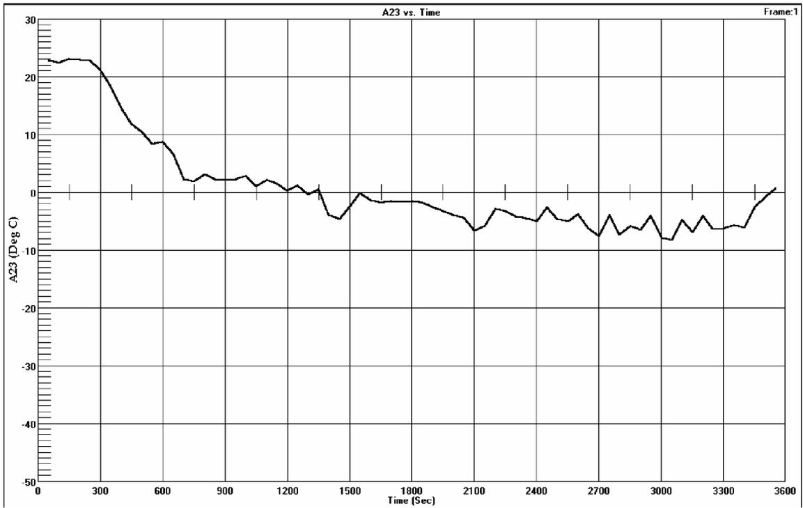
All frames are in sequence. Each frame represents one hour. The first frames show ambient conditions and ramping down to -40°C for the initial pre-soak with the EUT de-energized prior to start of test.
