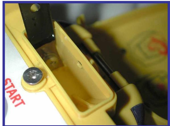
Water filled antenna storage well of
