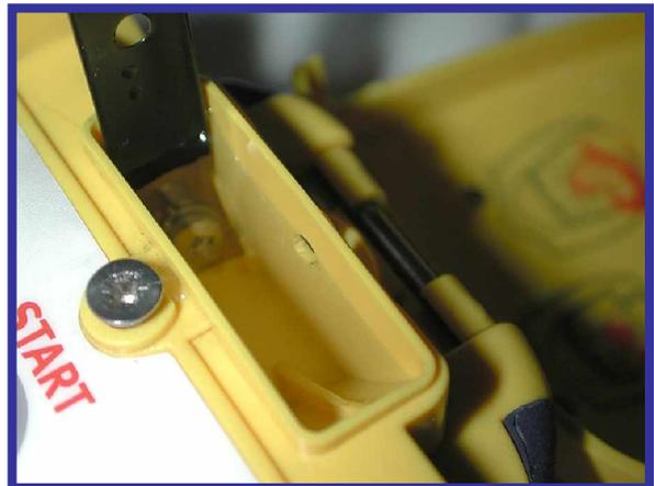
Water filled antenna storage well of
