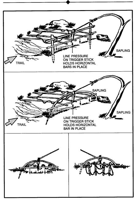
Figure 8-11. Treadle spring snare.
