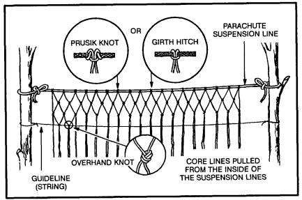
Figure 8-19. Making a gill net.
