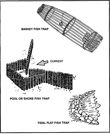
Figure 8-21. Various types of fish traps.
