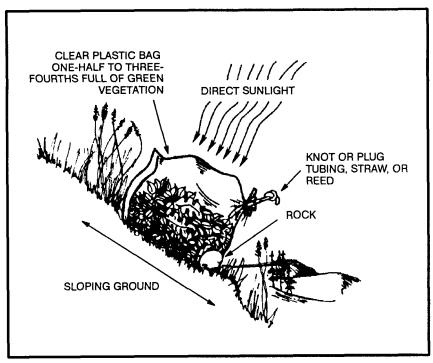
Figure 6-6. Aboveground solar water still.
