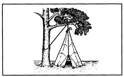
Figure 5-6. No-pole parachute tepee.
