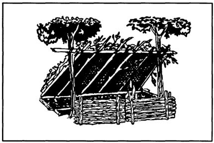
Figure 5-9. Field-expedient lean-to and fire reflector.
