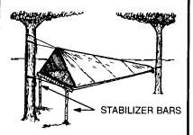
4 Drape the remaining three gores over the awning line and tuck the sixth gore into the shelter. Prop forked branches under the spreader bar to stabilize the shelter.
