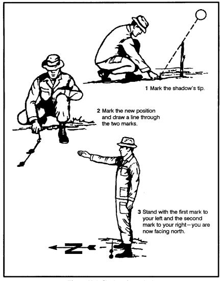
Figure 18-1. Shadow-tip method.
